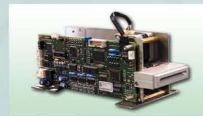
ENC2K1/R Magnetic reader encoder
